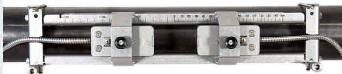
Measurement with transducers mounted with the portable Variofix VP
